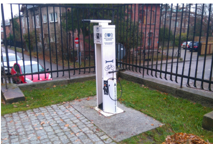
Fig. 5. Self-service repair station for bicycles. Fot.: K.Janiszevska
